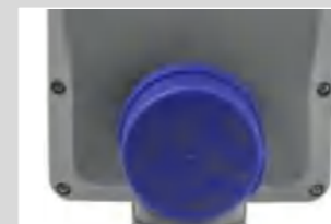
Photocell sensing: Lights off during the day and lights up at night.
